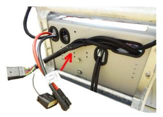
4. Plug the light harnesses to the lift frame harness (5) and secure them under the pump cover. Attach the power unit leads from the lift frame harness (5) to the coils. (Drawing 3,4,5)
