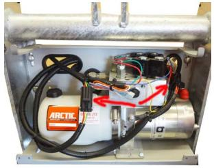
5. Mount solenoid (10) and relays (1) to metal surface close to the driver (as show on the picture) bending bracket if necessary. NOTE: <u>Solenoid must be well grounded</u> in order to function properly. (Drawing 1)
