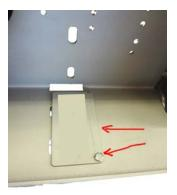
If M3493 is installed On Hi Boy Lift frame, install spacer plate and secure it with 1/4" bolt.
